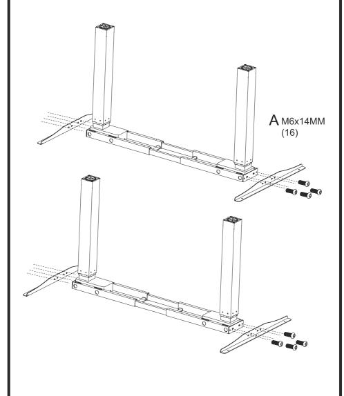
4. Assembly the middle inner fix brackets on four legs
