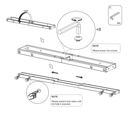
2. Assembly the motor height adjustable legs.
